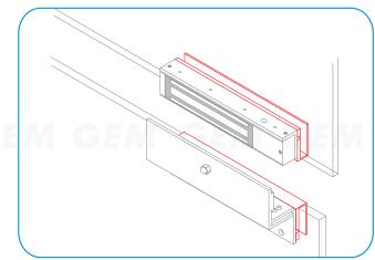
Suitable for use with frameless glass doors and the glass wall, After the door installs with the U-bracket, the door will become a single swing (inward opening) door. The glass thickness is 14 mm maximum The diagram shows the LZ-300 bracket installation instructions.
